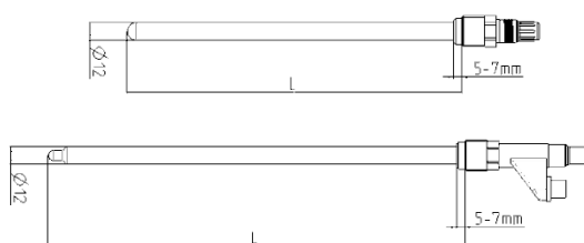
Figure 7: Sensor filled with gel (top), sensor filled with liquid (bottom)
