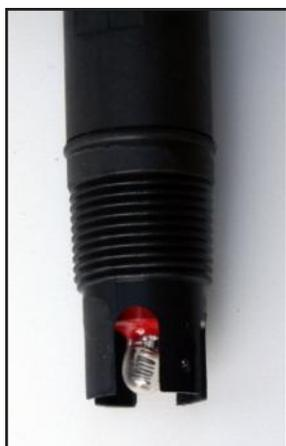
In addition, as REFEX possesses an inherently higher junction impedance than most traditional reference electrodes the increase in impedance due to fouling has a much lower effect even when the fouling is advanced.
