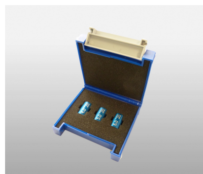
EXcap 110 - set of optical reference filters
