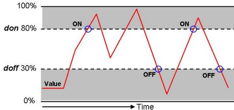
If  $d_{on}$  equals  $d_{off}$ , the output is switched on once the measured value exceeds the switching value  $d_{on} + d_{off}$  and is switched off once the measured value falls below the switching value  $d_{on} + d_{off}$  again.
