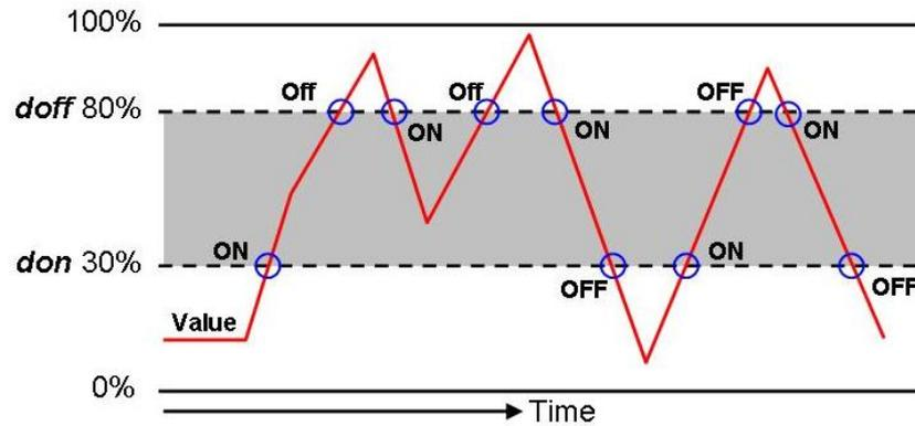
If  $d_{on}$  is higher than  $d_{off}$ , the output is switched on once the measured value exceeds  $d_{on}$ . The product is switched off only when the measured value falls below  $d_{off}$  (hysteresis function).
