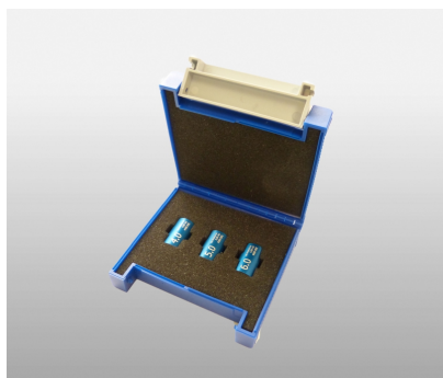
EXcap 110 - set of optical reference filters
