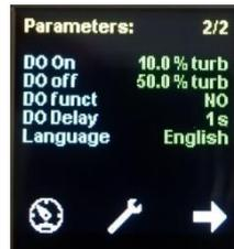
To return to the display, press the dial symbol or wait for 30 seconds without making any input or touching the display.
