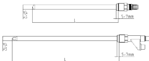
Figure 9: Sensor filled with gel (top), sensor filled with liquid (bottom)
