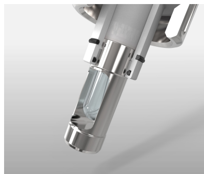
Sealing system of the EXtract825 with the reliable PTFE scraper.
