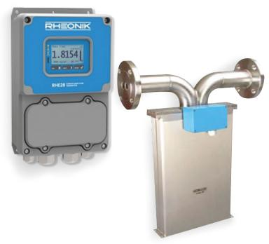
For any upgrade to a combustion process that includes flexible fueling, Coriolis flowmeters offer the best solution for the fuel flow measurement. Coriolis flow meters accurately and reliably measure the flow and density of liquid fuels, even when the fuel feed is switched from one liquid to another.
