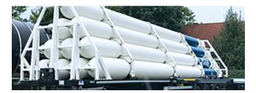
Few filling stations have pipelines supplying them with Hydrogen 24/7; for those who do not, it falls to trucks with high-pressure tube trailers to deliver hydrogen to local storage at filling stations. In order to control and account for the quantity of gas being delivered to local sites, each truck is equipped with a flow meter that totalizes the amount of each gas transfer.
