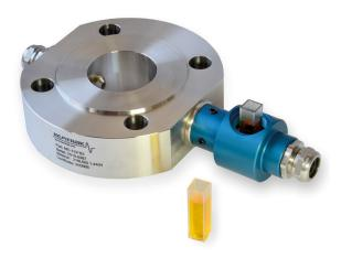
The Kemtrak DCP007-NIR process analyzer is a high performance fiber optic coupled near-infrared (NIR) photometer for high resolution, real time, inline concentration measurement.
