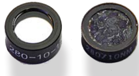
left: Optical filter used on a Kemtrak DCP007-UV photometer right: Eroded optical filter from a traditional hot mercury vapor lamp photometer
