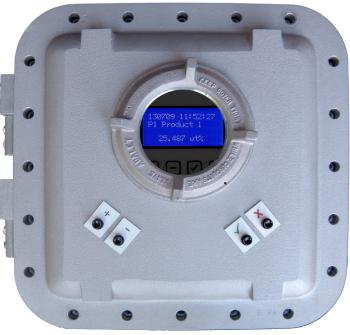
parts to perform the measurement. Fiber optics are ideally suited for use in explosive environments as they only allow transmission of ultra-low power cold light supplied from a high performance LED light source within the instrument.
