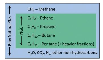
Gas processing plants separate methane (C1) from the raw natural gas stream for distribution around the country in natural gas pipelines. The remaining products (C2+) are typically transported in an NGL pipeline for further processing at other facilities such as refineries.
