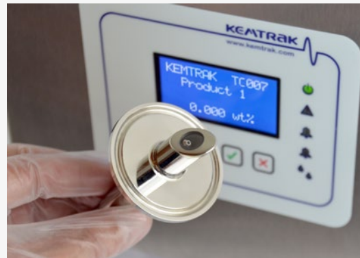
Kemtrak TC007 Back Scatter Insertion Turbidimeter
