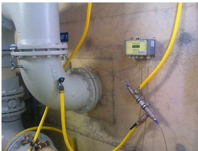
A Kemtrak DCP007 photometer with a long pass flowcell installed for evaluation purposes
