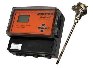
A typical system comprises of a sensor and a controller connected via special cables. The sensor probe is installed in the process such that it sits above the liquid level. When the foam level reaches the probe, the controller will begin dosing chemical using a configured strategy until the foam level subsides.
