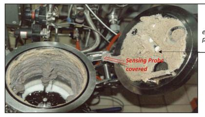
A small batch reactor still operating efficiently with the probe covered and totally hidden!
